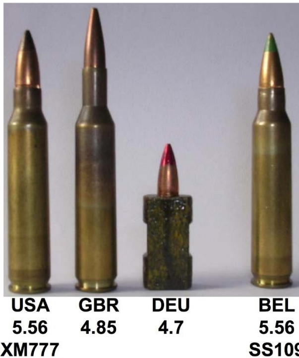
Figure 54 - The XM777 and the other cartridges considered in the NATO trials.
