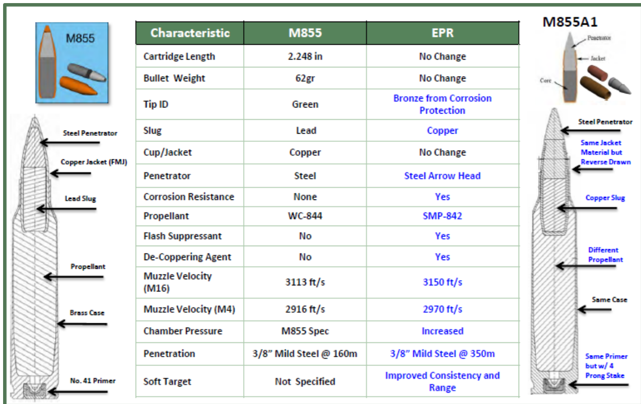
Figure 49 - Comparison of the changes from the M855 to the M855A1, from the report, M855A1 Enhanced Performance Round (EPR) Media Day
