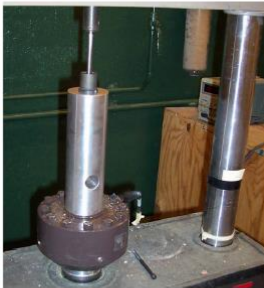
Figure 50 - The testing set up used in the Push Test report that warned of some of these issues with the M855A1 back in 2007.
