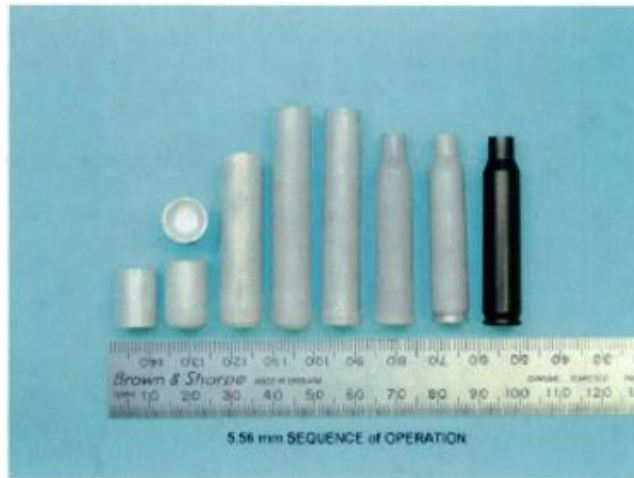
Figure 44 - Aluminum cases in the various stages of being formed from the report, Aluminum Cartridge Case Concept.
