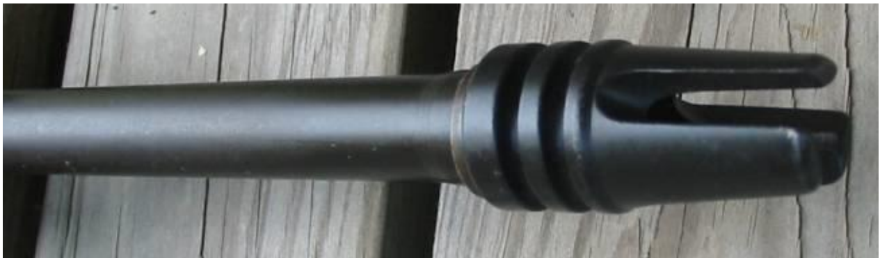
Figure 18 - The three prong design was eventually replaced by the A2 "Birdcage" design.
