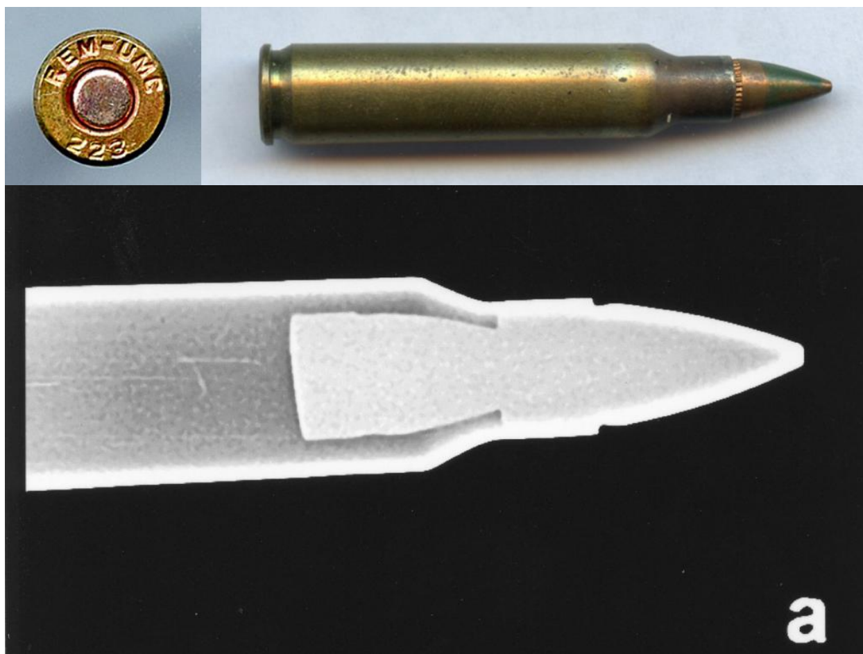
Figure 9/10 - While externally the duplex .223 rounds looked similar to a standard round, X-Rays show the dual slug design.
