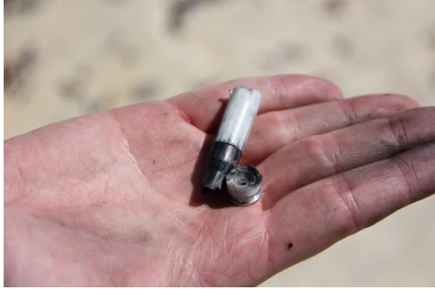
Figure 28 - Example of a polymer cased .308 round failing, causing a "Ka-BOOM".
